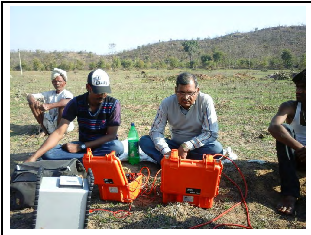
Fig. 5.1 Conducting Resistivity survey in Chhattarpur distt. (M.P.)
